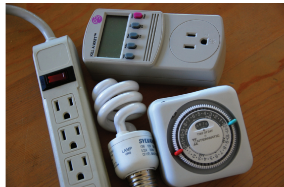
Figure 5. Home energy saving and monitoring devices: compact fluorescent light bulb, power strip, timer, watt meter.
